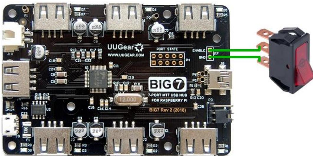
You can also connect the ENABLE pin to a GPIO pin in Raspberry Pi, and control the USB ports' power by setting the GPIO pin high/low.
