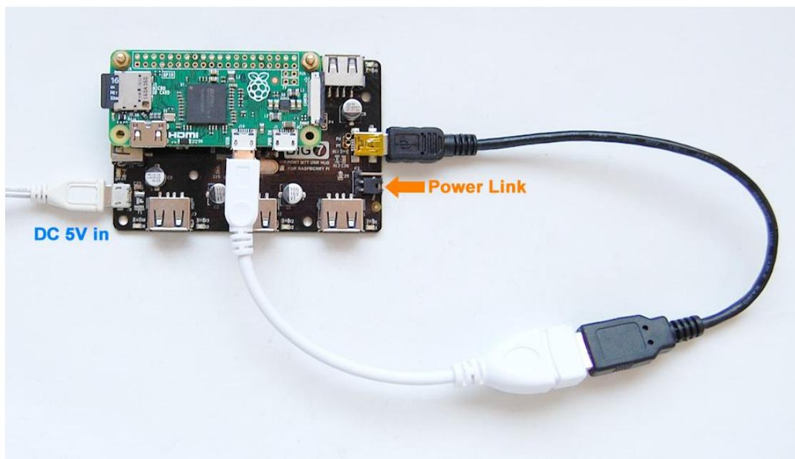
If you don't want the back-powering, just put the jumper to the other side and connect two power supplies to USB hub and Raspberry Pi Zero accordingly.
