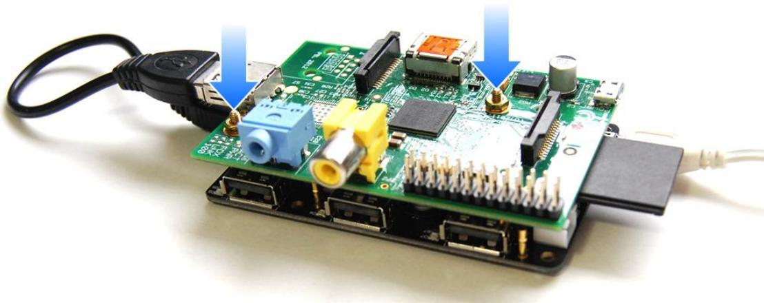
Use the USB - mini USB cable to connect the USB port on Raspberry Pi and the mini USB port on the USB hub and then it will be ready to work.
