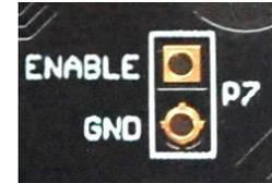
The ENABLE pin is pulled up (to 3.3V) by default. The power of USB ports will be cut when the ENABLE pin is shorted to the GND (ground) pin. By cutting the power of USB peripherals, they can not draw any current from the USB hub and doing so can save the power consumption. This would be very useful if your project is running with very limited power source (battery, solar panel etc.).
