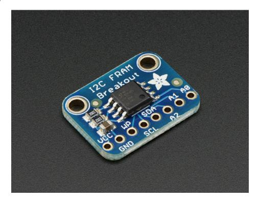
You're probably familiar with SRAM, DRAM, EEPROM and Flash but what about FRAM? FRAM is 'ferroelectric' RAM, which has some very interesting and useful properties. Unlike SRAM, FRAM does not lose the data when power is lost. In that sense it's a durable storage memory chip like Flash. However, it is much faster than Flash - and you don't have to deal with writing or erasing pages.
