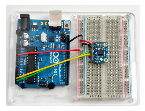
• Connect **Vcc** to the power supply, 3V or 5V is fine. Use the same voltage that the microcontroller logic is based off of. For most Arduinos, that is 5V
