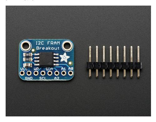
This particular FRAM chip has 256 Kbits (32 KBytes) of storage, interfaces using I2C, and can run at up to 1MHz I2C
