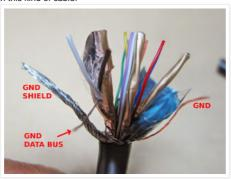
Now, this is a smaller diameter (it was Micro HDMI before I cut it) cable with only 15 threads. This cable has 5 data shields but there are no GND lines in them! There is not GND shield, just a wrapping that was cut before taking the picture. The HDMI connectors are put to GND. This cable does not work out of the box with the Raspberry Pi Camera extension kit.
