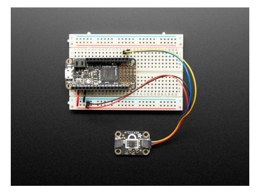
Please note the I2C address is fixed at 0x60 and according to Microchip, you should use this at higher I2C speeds like 400KHz if other devices are on the I2C bus, to avoid some I2C bus contention (much like the datasheet, this is not documented anywhere yet).
