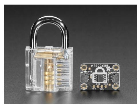
The ATECC608 is the latest crypto-auth chip from Microchip, and it uses I2C to send/receive commands. Once you 'lock' the chip with your details, you can use it for ECDH and AES-128 encrypt/decrypt/signing. There's also hardware
