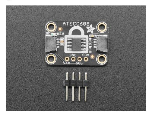
To make working with the ATECC608 as easy as possible, we've put it on a breakout PCB with the required support circuitry and SparkFun qwiic (https://adafru.it/Fpw) compatible STEMMA QT (https://adafru.it/Ft4) connectors. This allows you to use it with other similarly equipped boards without needing to solder. This chip will work with 3.3V or 5V power/logic micros, so it's ready to get to work with a range of development boards.
