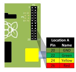
With the Pi-Stop fitted in the correct position you can now power up your Raspberry Pi.
