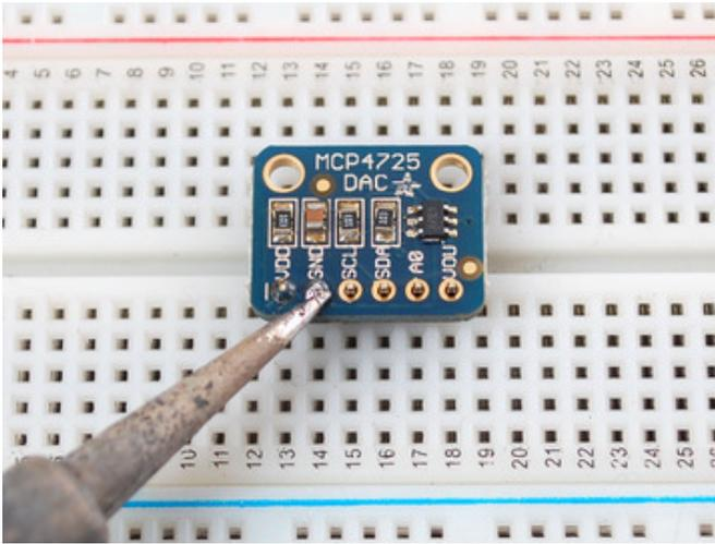
Solder each pin using a soldering iron and solder, to make solid connection on each pin.
