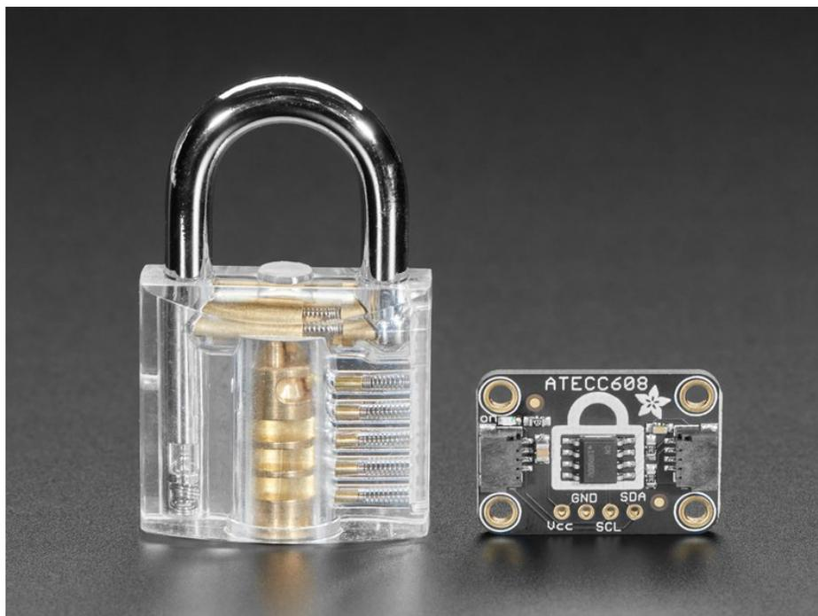
The ATECC608 is the latest crypto-auth chip from Microchip, and it uses I2C to send/receive commands. Once you 'lock' the chip with your details, you can use it for ECDH and AES-128 encrypt/decrypt/signing. There's also hardware
